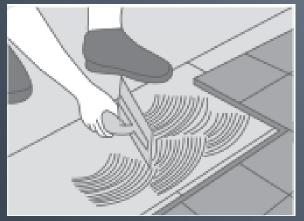
Apply tile adhesive onto the sheet using a notched trowel. Refer to adhesive manufacturer's instructions.
